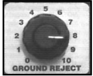
Figure 9. The GROUND REJECT control consists of a coarse-adjustment knob on top of a fine-adjustment knob.
